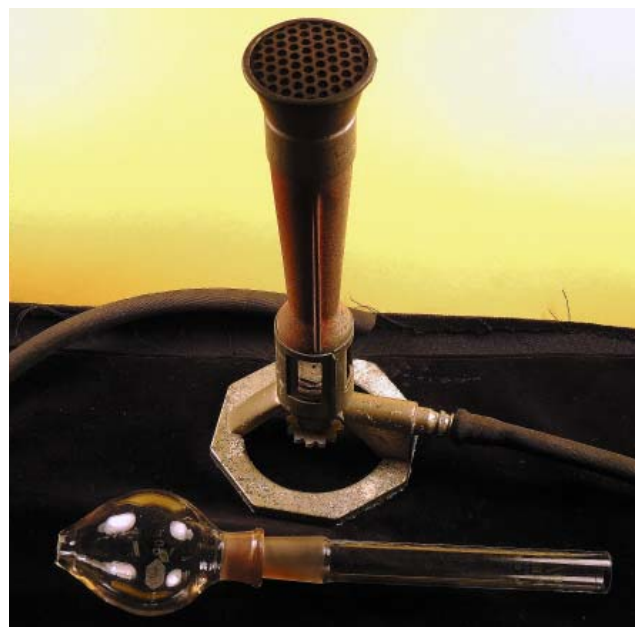
Text-fig. 7. Simplified Teichert method. “Air drive” is simply by blowing into the end of the drying tube. This method works best when using a large (Fisher) burner and constantly rotating the tube while heating.
