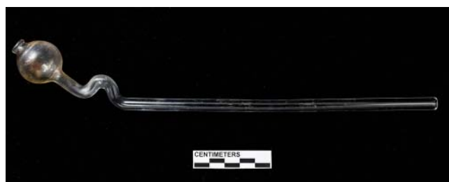
Text-fig. 5. The Michigan tube. This version of a drying tube is bent to trap moisture from the breath from reaching the heated \text{NH}_4\text{Cl} . These tubes were made by a glass blower at the University of Michigan, Ann Arbor. Illustration courtesy Dan Fisher, Director, Museum of Paleontology, Univ. of Michigan.
